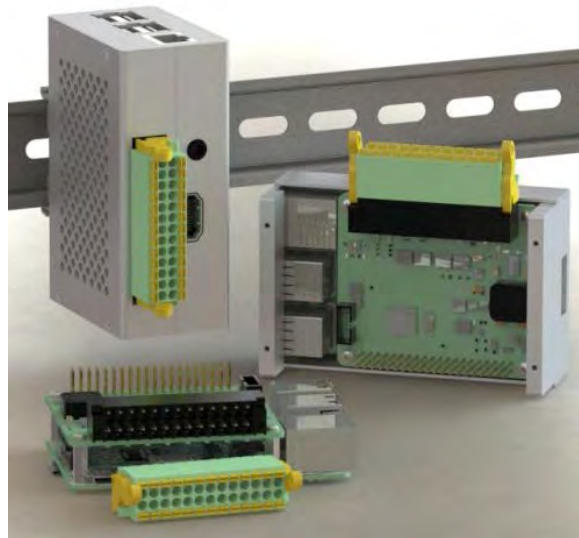
Figure 55 Monarco HAT plain board and with housing
